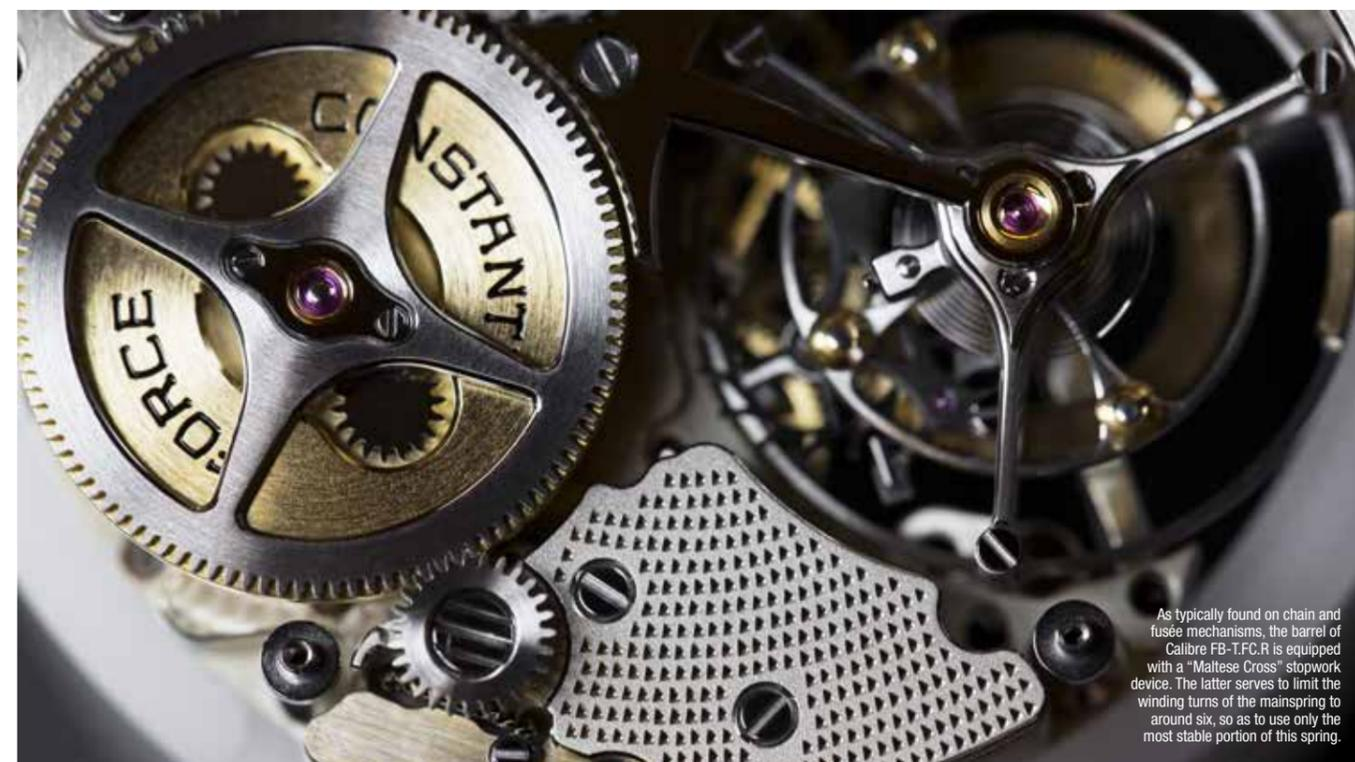
As typically found on chain and fusée mechanisms, the barrel of Calibre FB-T.FC.R is equipped with a "Maltese Cross" stopwork device. The latter serves to limit the winding turns of the mainspring to around six, so as to use only the most stable portion of this spring.
